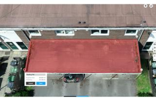
The 3D models are photographic in detail, allowing up close inspection. Geo-tagged data inputs and intelligent photogrammetry algorithms mean that the model is scaled accurately. Yorkshire Housing can take line, area or volume measurements at any point on the model with centimetre level precision.
