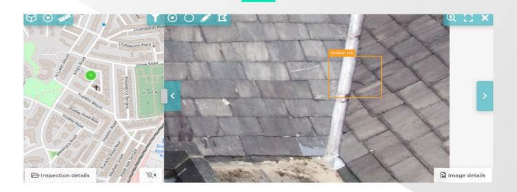
A separate browser based portal called Scopito is used to store, organise and inspect the hundreds of detailed photographs taken by the drones. Annotations, severity, categories and locations of any defects or points of interest can be added and subsequently filtered and searched.
