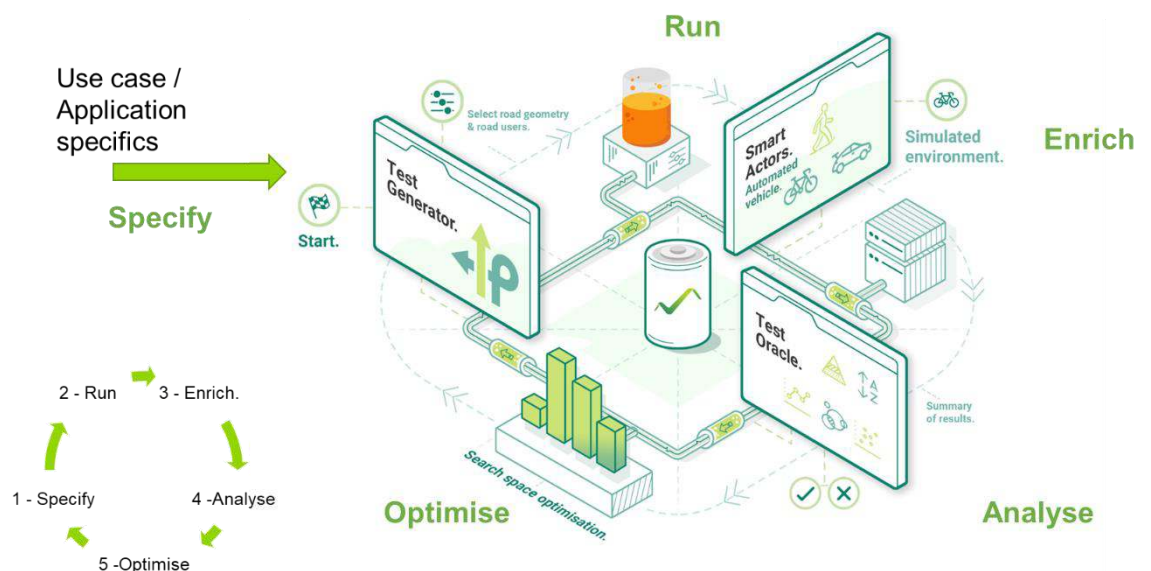
Figure 33: Illustration core test execution process within the VeriCAV project
